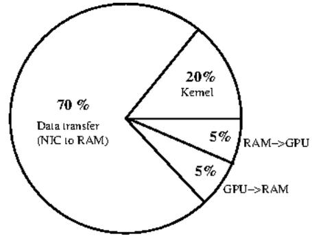
**Figure 2.** Time budget of data processing on GPU.
