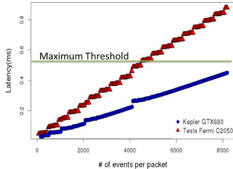
**Figure 8.** Total latency (including data transfer and computing).
