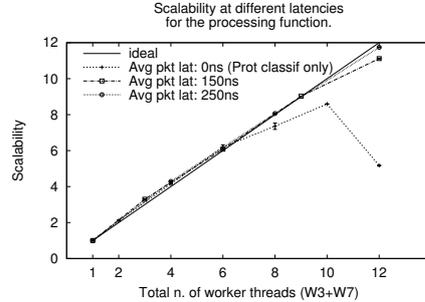
**Figure 4.** Scalability increasing packet processing computation time.
