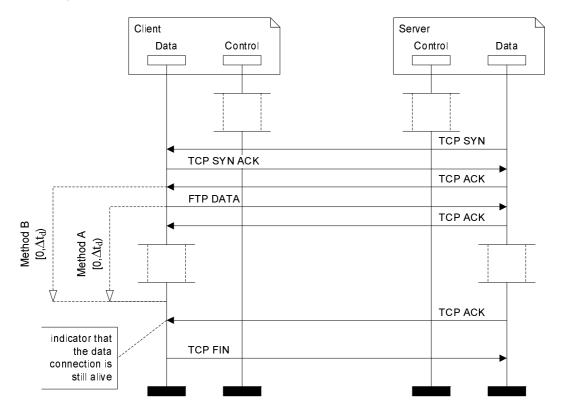
Figure 3: Diagram of Events for FTP upload, active mode, includes both Data transfer start methods A and B
