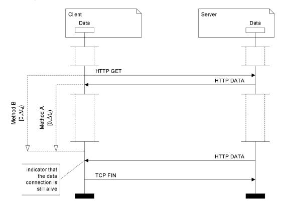
Figure 5: Diagram of Events for HTTP download, includes both Data transfer start methods A and B
