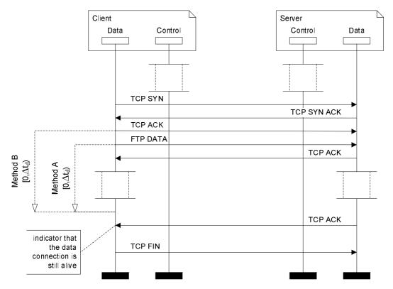
Figure 4: Diagram of Events for FTP upload, passive mode, includes both Data transfer start methods A and B
