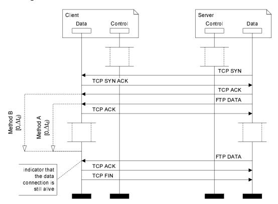
Figure 1: Diagram of Events for FTP download, active mode, includes both Data transfer start methods A and B
