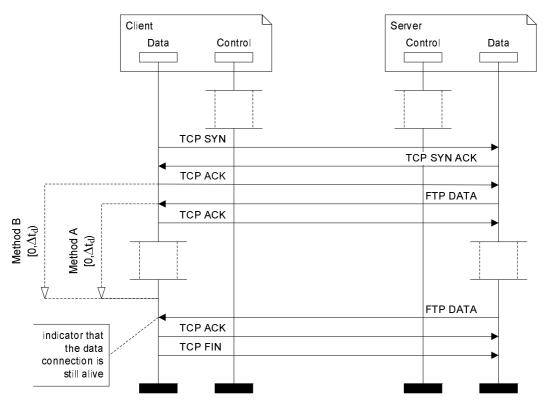
Figure 2: Diagram of Events for FTP download, passive mode, includes both Data transfer start methods A and B
